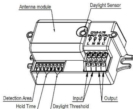
By selecting the combination on the DIP switch, sensor data can be precisely set for each specific application.
