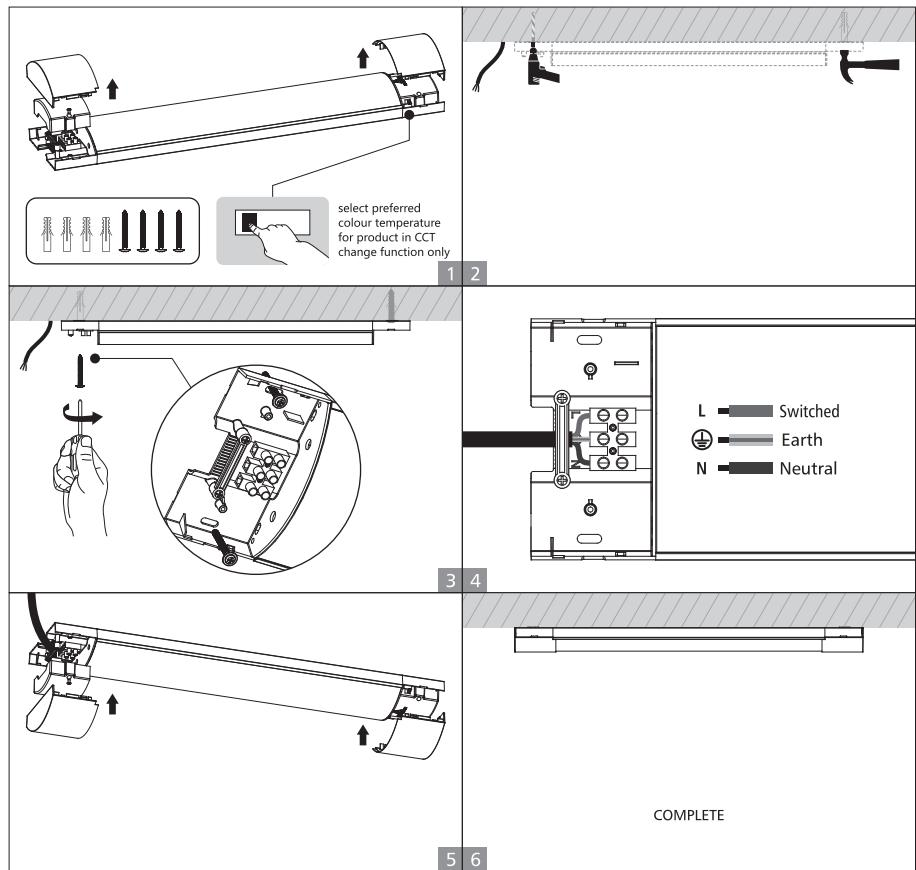
**Note:** This product is colour switching, please remember to select the correct colour prior to the final assembly of the light.
