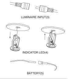
ENSURE ELECTRICAL SUPPLY AND BATTERY CONNECTION IS DISCONNECTED/ISOLATED BEFORE COMMENCING INSTALLATION OR ANY MAINTENANCE WORK. HIGH VOLTAGE COULD BE PRESENT AT THE OUTPUT CONNECTION IF THE BATTERY IS NOT DISCONNECTED.
