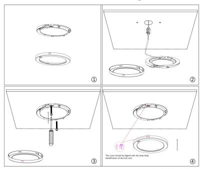
I.Take off surface cover 2.Connect power cable with terminal 3.Use screws fixing light onto roof through light housing holes
