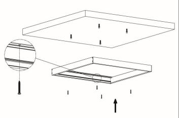
3. Fix semi-finished frame onto ceiling with screw(Concrete ceiling requires plastic anchor)
