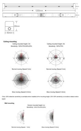
Default Setting of sensor: Detection Area: 100%, Hold Time: 5S, Stand-by period: 0s, Stand-by dim level: 10%, Daylight sensor: Disabled
