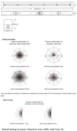
Stand-by period: 0s, Stand-by dim level: 10%, Daylight sensor: Disabled
