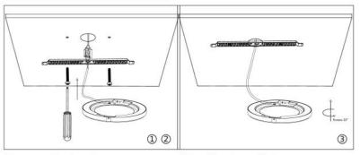
1.Connect power cable with terminal 2.Fix bracket onto ceiling with screws 3.Twist on light to tighten it with bracket
