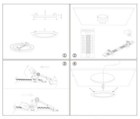
I.Adjust springs to suitable size position according to ceiling cut-out 2.Twist on bracket into light; 3.Connect power cable with terminal4.Pull up springs, install light into ceiling cut-out
